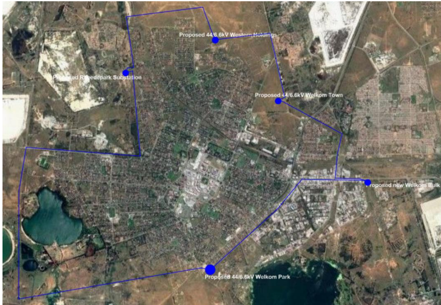
Figure 7-13: Proposed Welkom 44kV Ring
